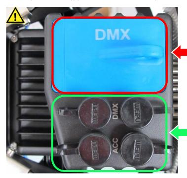
The 5pin XLR connector connectors located under the blue rubber cap ARE NOT WATERPROOF!
