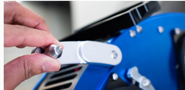
Carefully retract spring loaded pin for attachment.
